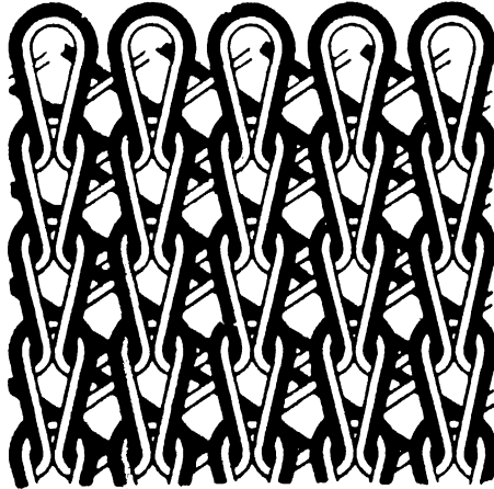
FIG. 26 MILANESE FABRIC ( WARP-KNITTING ) WITH SILK LAP
